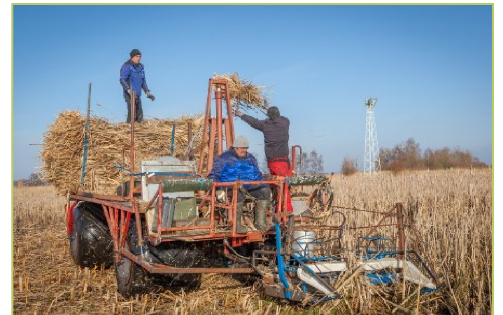
Figure 2 Cattail mowing test with a Saiga, a reed harvest machine adapted to harvest of reed bundles (photo: T. Dahms)
